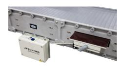
The Metal Detector Module is an ideal system for inspecting plastic scrap for metal contaminants as scrap is conveyed to grinders. Early detection of metal can prevent severe damage to grinder blades subsequent fouling injection systems and molded plastic products (where product liability issues could result).
